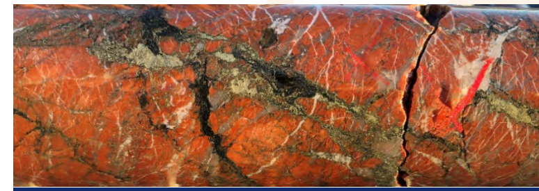
Chalcopyrite and pyrite fracture infill hosted by a mylonitized Pegmatite – HTODD001, 212.6m
