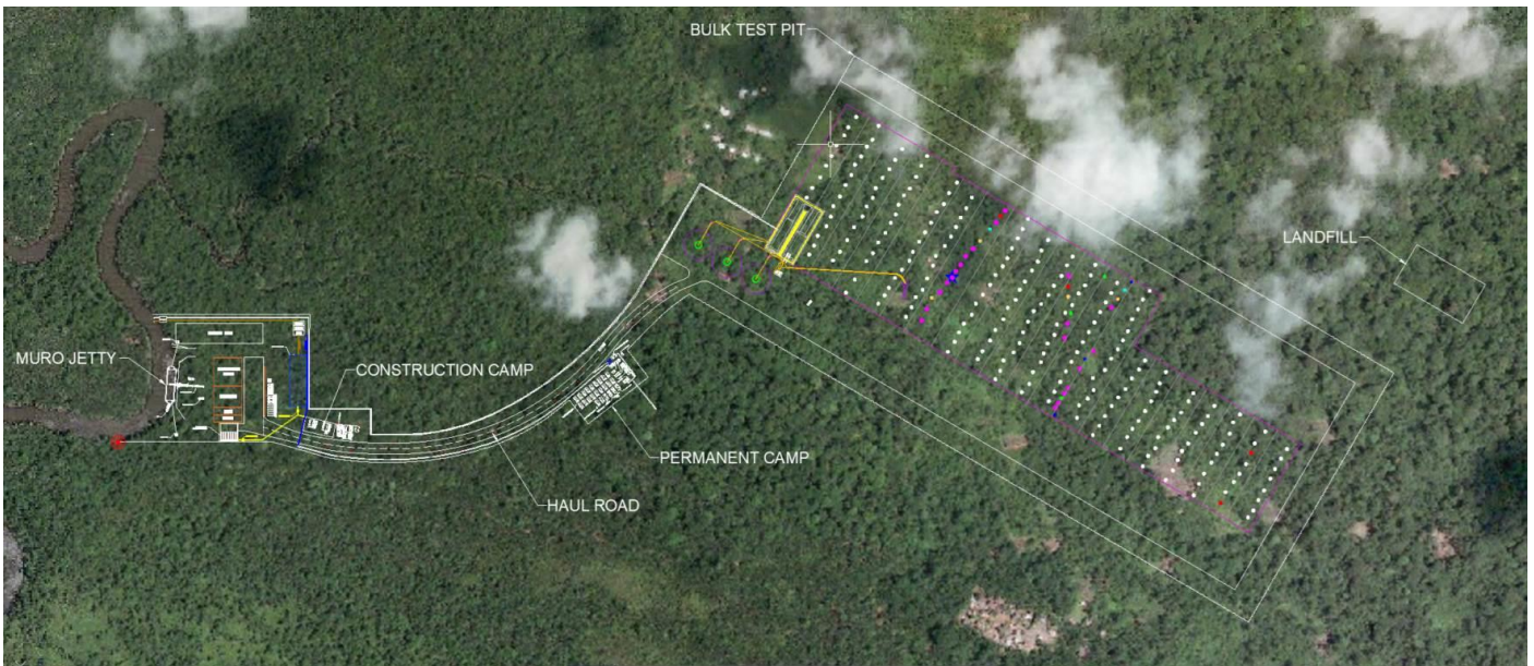
Figure 4: Orokolo Bay pilot plant, bulk sample pit layout and loading point on Muro River
