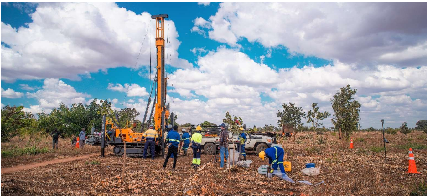
Figure 9: Core drilling (push tube) in action at Kasiya
