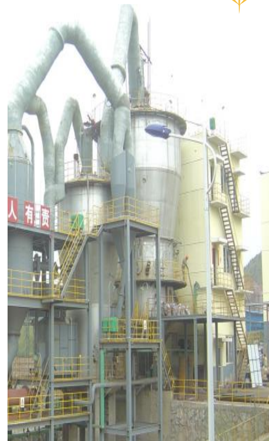
BGRIMM 200tpd Two-Stage Fluidized-Bed Roaster
