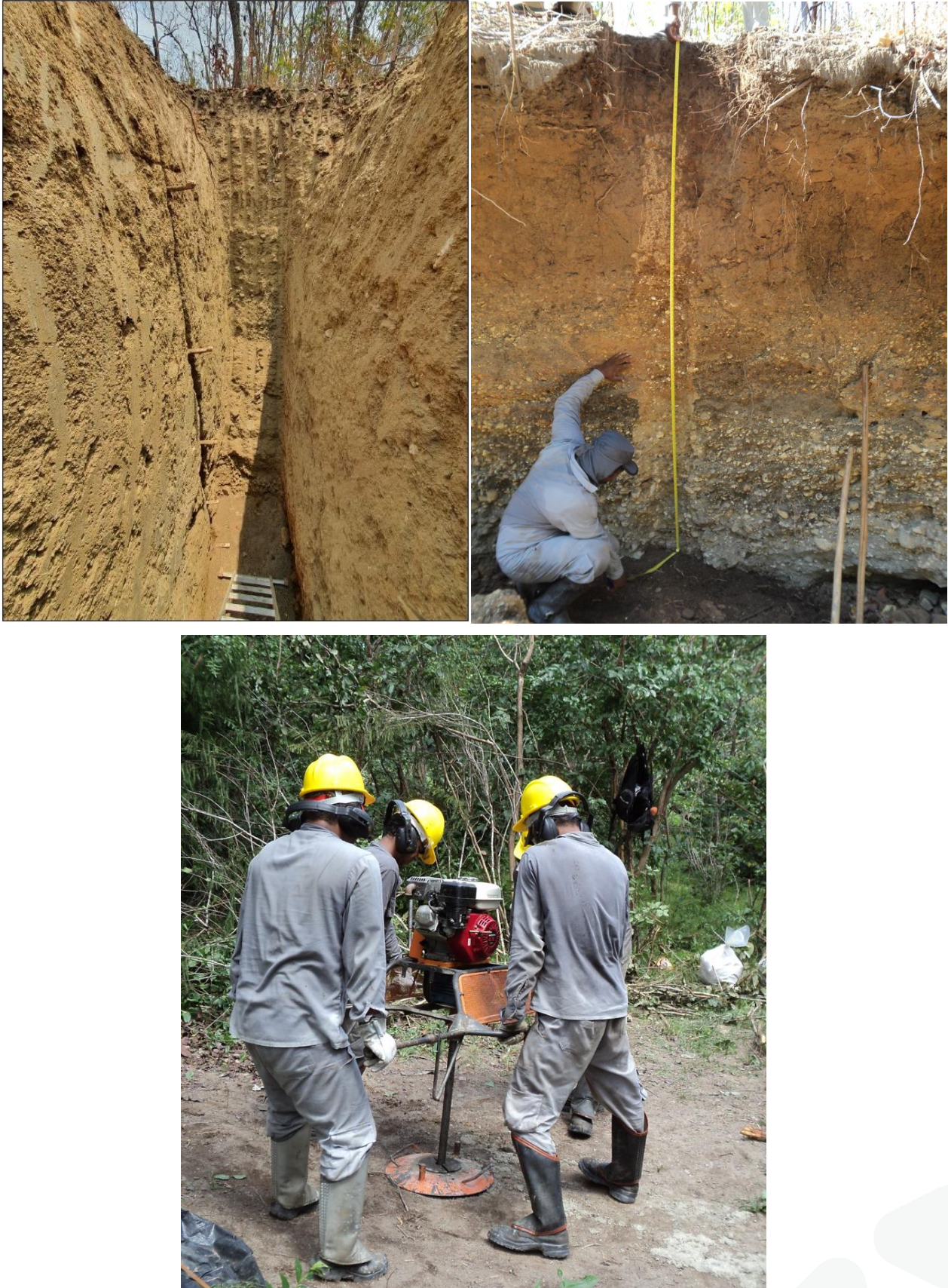
Figure 2: Photos from Mata Azul - Bluebush Exploration. Top left is an excavated pit with sampling intervals marked on left wall. Top right is measuring the thickness of an alluvial bank prior to sampling and the lower photo shows the handheld auger drilling.
