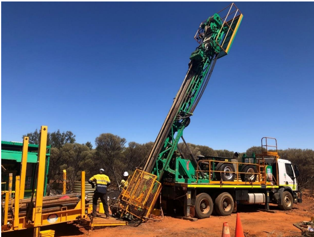
Photo 1 – Diamond drill rig commencing drill programme at the Leinster Nickel Project
