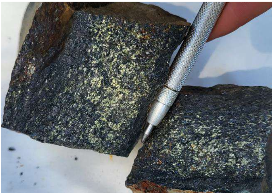
Figure 6: Massive magnetite & abundant disseminated discordant chalcopyrite, (sample GYTR074 494105 East/6597034 North in SWEREF99 TM = EPSG3006). pXRF analysis 1.45% Cu, equivalent to approximately 4% chalcopyrite.
