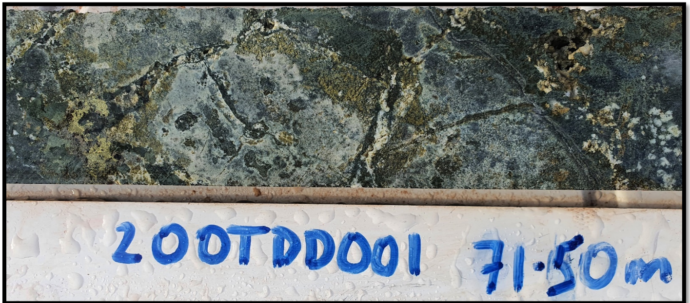
Figure Three: Photographs of HQ drill core from hole 200TDD001. The top photo shows altered and weakly brecciated basalt and the bottom photo shows chalcopryite and associated carbonate (white) and epidote-chlorite (green) alteration. The width of the is core 63mm.
