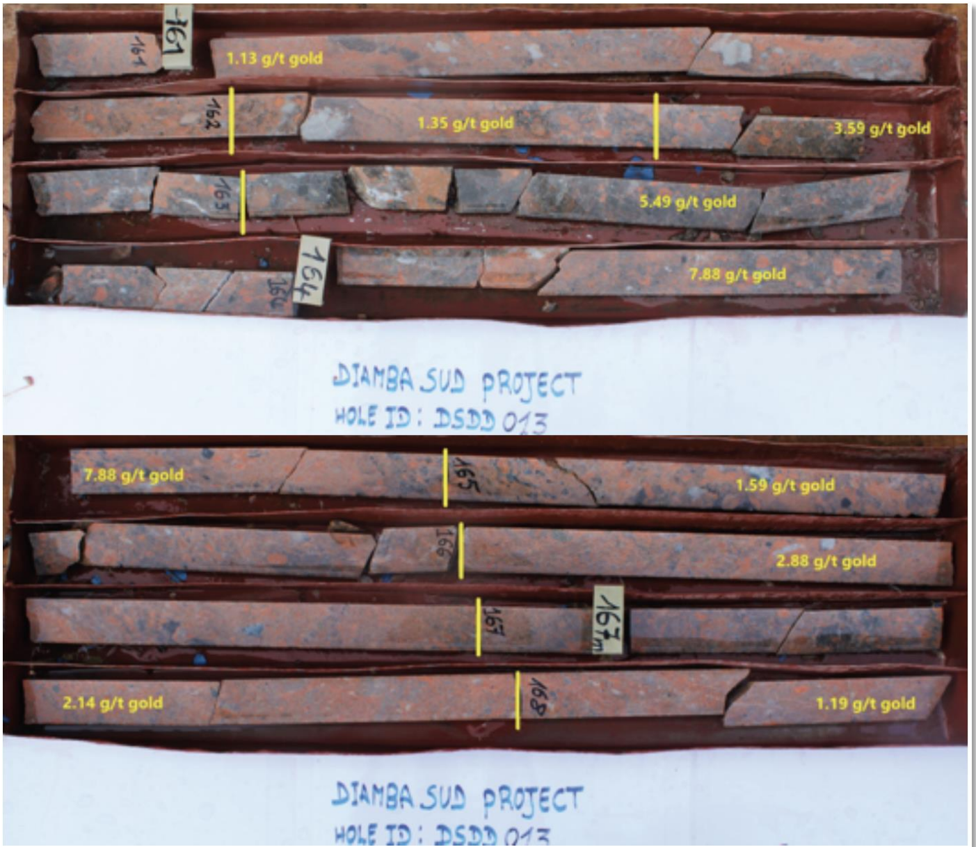
Figure 7: Area A, hole DSDD013 intersection from 161m to 168.5m showing intense albite-carbonate-quartz alteration. Brecciated section 161-168.6 marks feeder structure. Mineralisation associated with coarse pyrite quartz stringers and minor visible gold.
