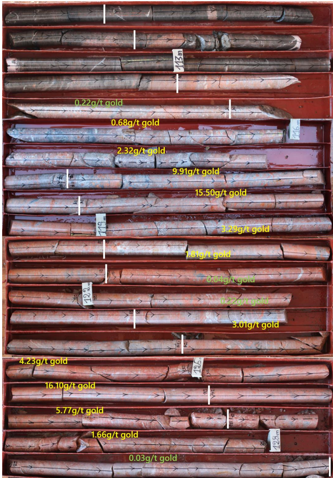
Figure 1: DSDD020 (111-128.96m) core showing mineralised zone on the SWF2 structure. Alteration and hydrothermal brecciation commences from 112.90m with strongly defined qtz-carb-pyr-tourmaline matrix in upper section. Strong albite-hem-Fe carb-qtz alteration throughout mineralised zone, with minor coarse pyrite agglomerations typically present in the high-grade NW-SE dilational fault.
