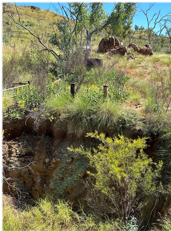
Figure 3. DeeJay Jude Prospect showing shallow workings in the foreground with outcropping copper mineralisation (green = malachite) and outcropping quartz goethite malachite mineralisation in the background.
