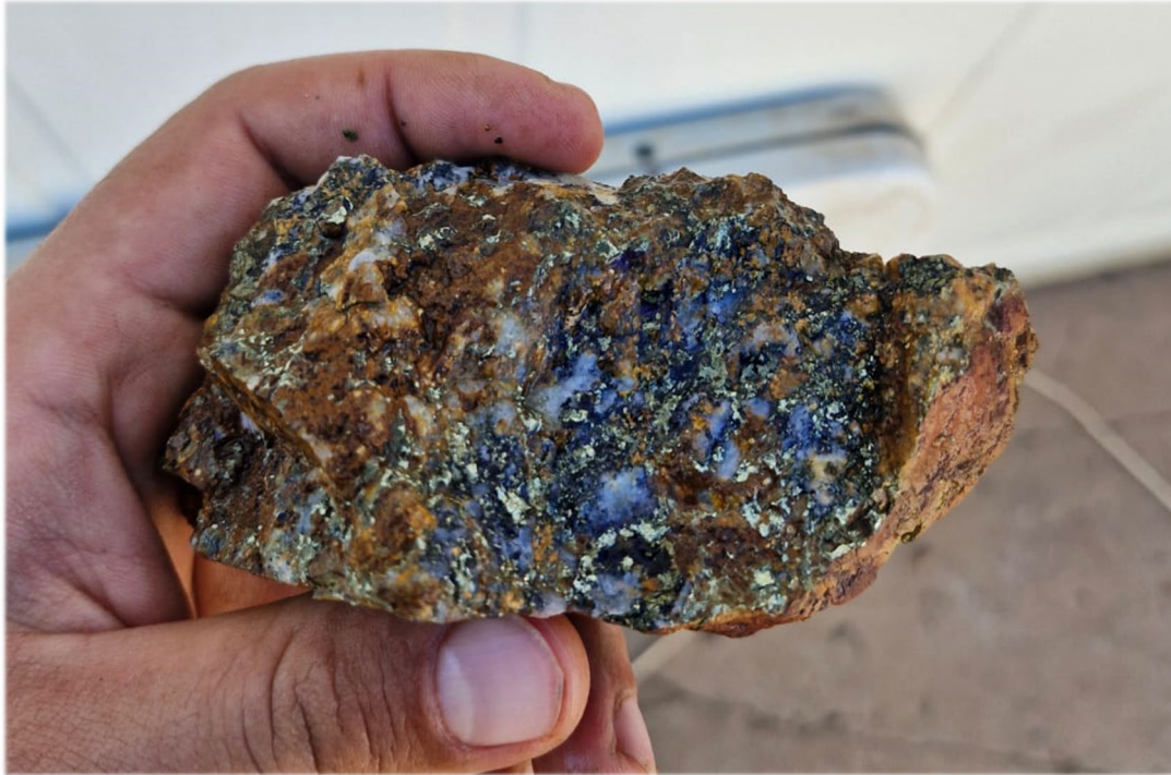
Figure 5. Hand Rock Chip Specimen from the Plus Prospect showing Mount Hope style quartz-chalcopyrite breccia mineralisation.
