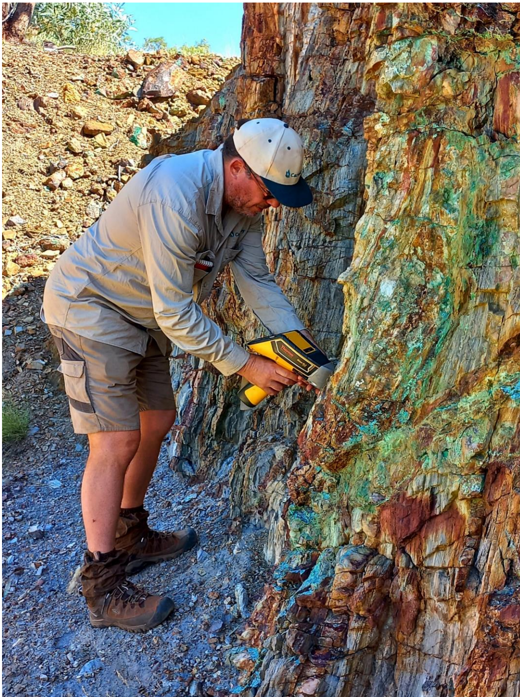
Figure 6. Carnaby Managing Director Robert Watkins completing due diligence with a portable XRF machine, analysing the outcropping malachite copper mineralisation (green mineral).
