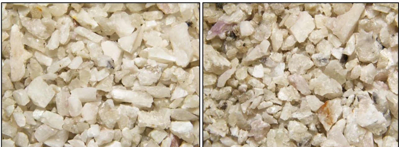
Figure 4 - HLS concentrate fractions grading ~6.0% Li 2 O (left) and ~5.5% Li 2 O (right)
