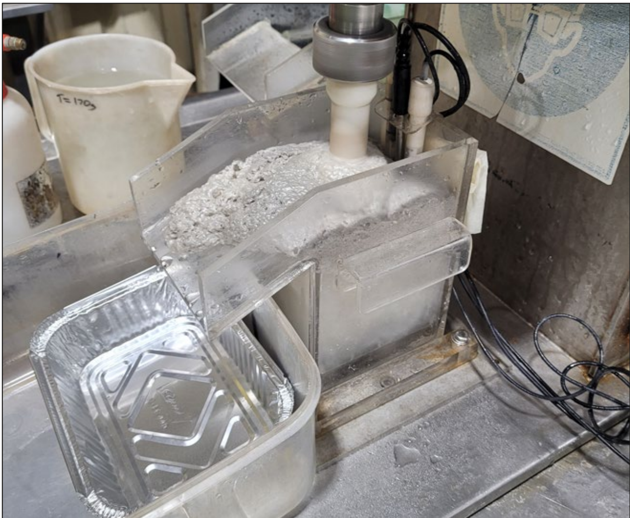
Figure 5 - Initial mineralised froth at the start of rougher flotation
