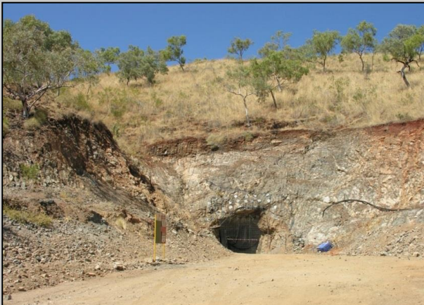
Panton portal from which bulk samples for metallurgical test work were taken
