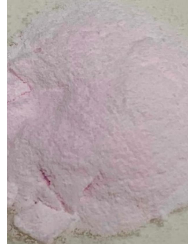
Oakover battery grade MnSO 4
