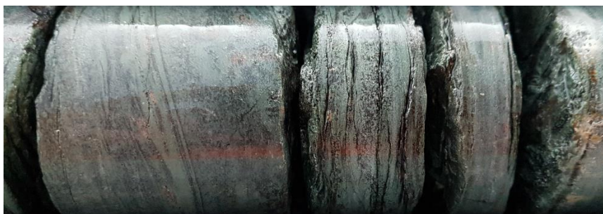
Figure 8. Black Allanite (REE bearing mineral with formula (Ce,Ca,Y,La)_2(Al,Fe^{+3})_3(SiO_4)_3(OH) ) within a Pyroxene Skarn - HMKPDD001, 155.5m.
