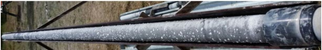
Figure 7 : Core well 270-06C visible gas emissions observed from core sample at depths between 277.75-280.75m
