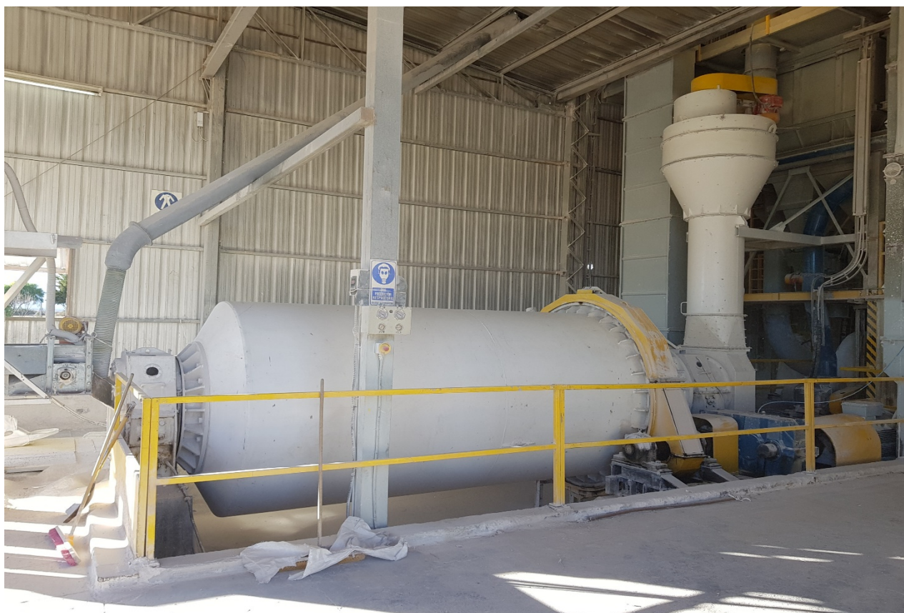
Figure 1: Ball mill for quartz and feldspar at an operating Plant in San Luis.
