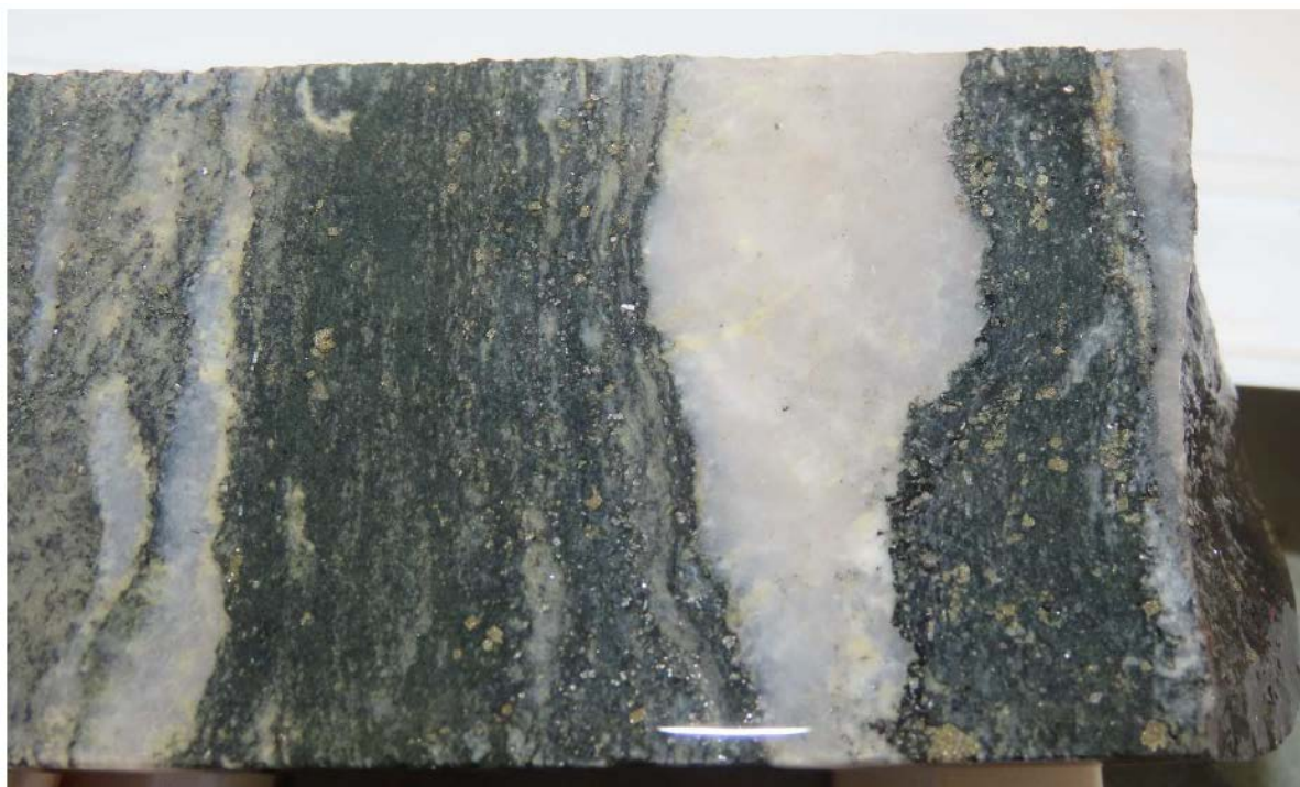
Figure 6: Core from 188.22-188.44m depth in diamond drillhole 20FNDD005 illustrates Type 1 ribbon quartz veins in strongly sheared mafic volcanics
