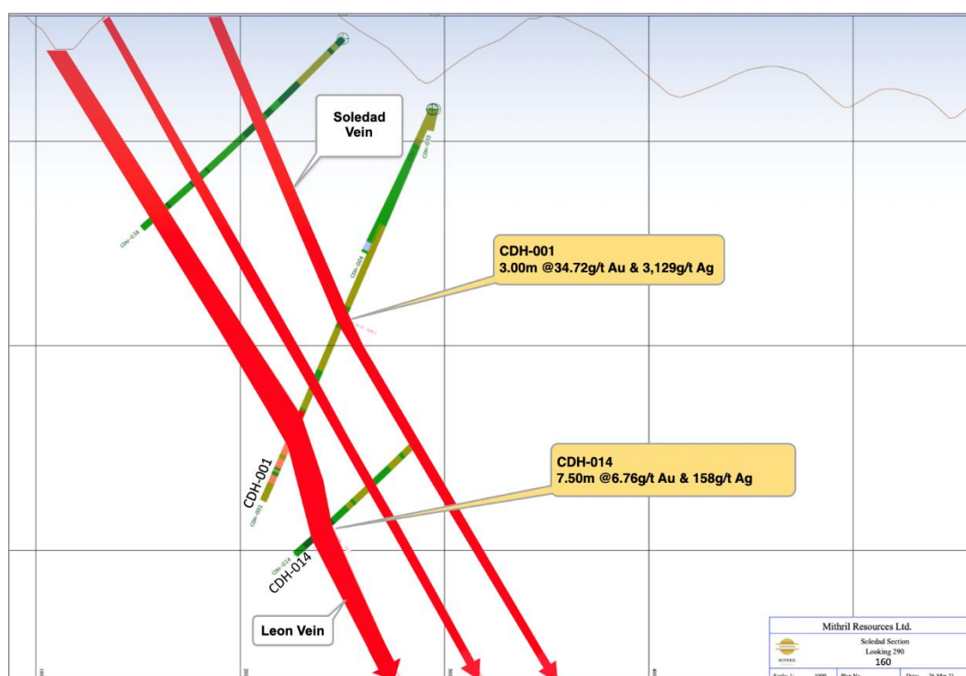
Figure 11 Cross Section 160 at La Soledad target showing hole CDH-001 and hole CDH-014
