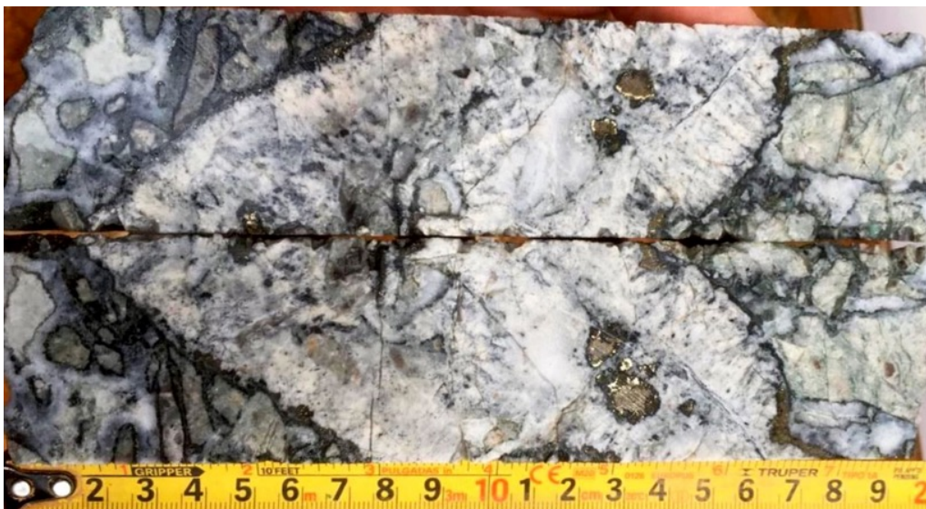
Figure 3: Two halves of cut NQ size core from hole CDH-077 472.1-472.3 metres with abundant visible gold
