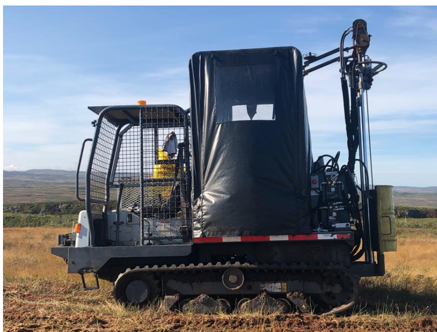
Figure 8: Power auger (rubber track-mounted “Winkie Rig” Mk2)
