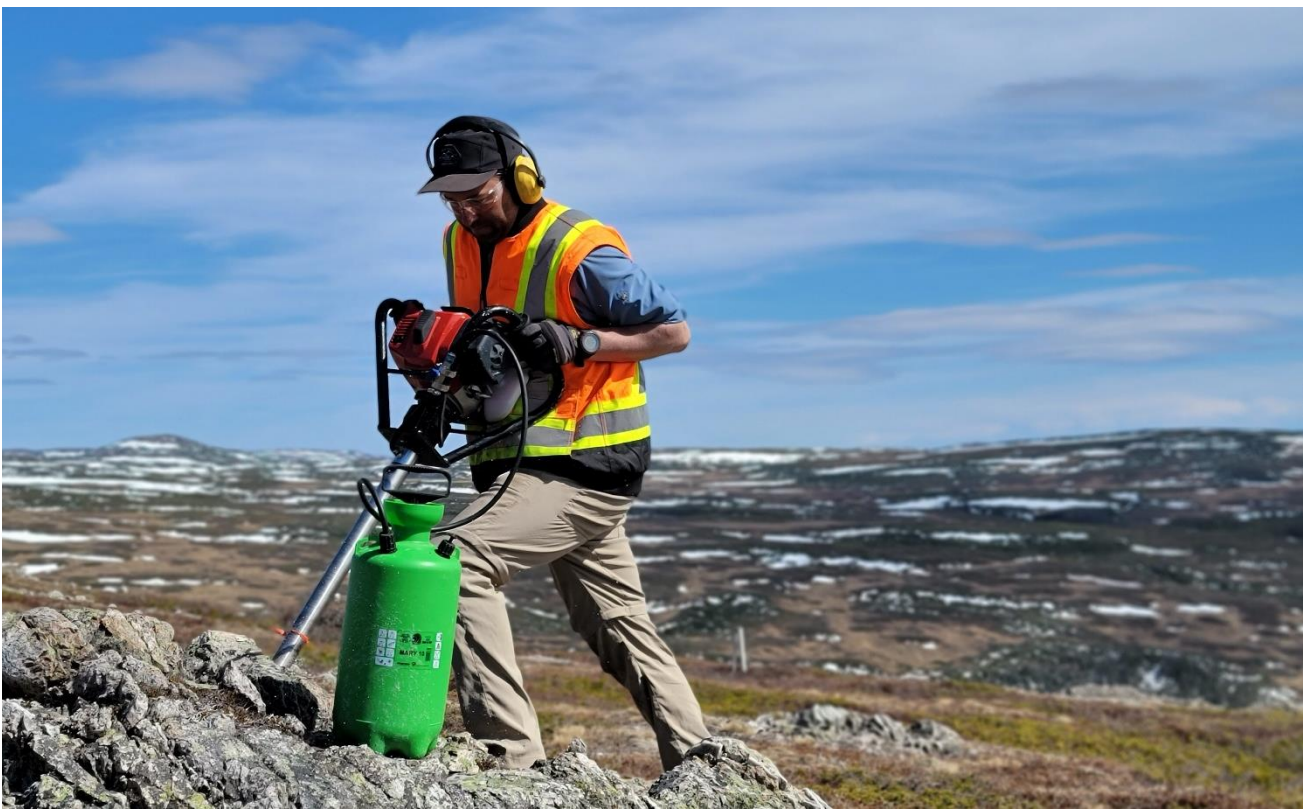
Figure 1: Hand-held power-auger drilling sampling outcrop
