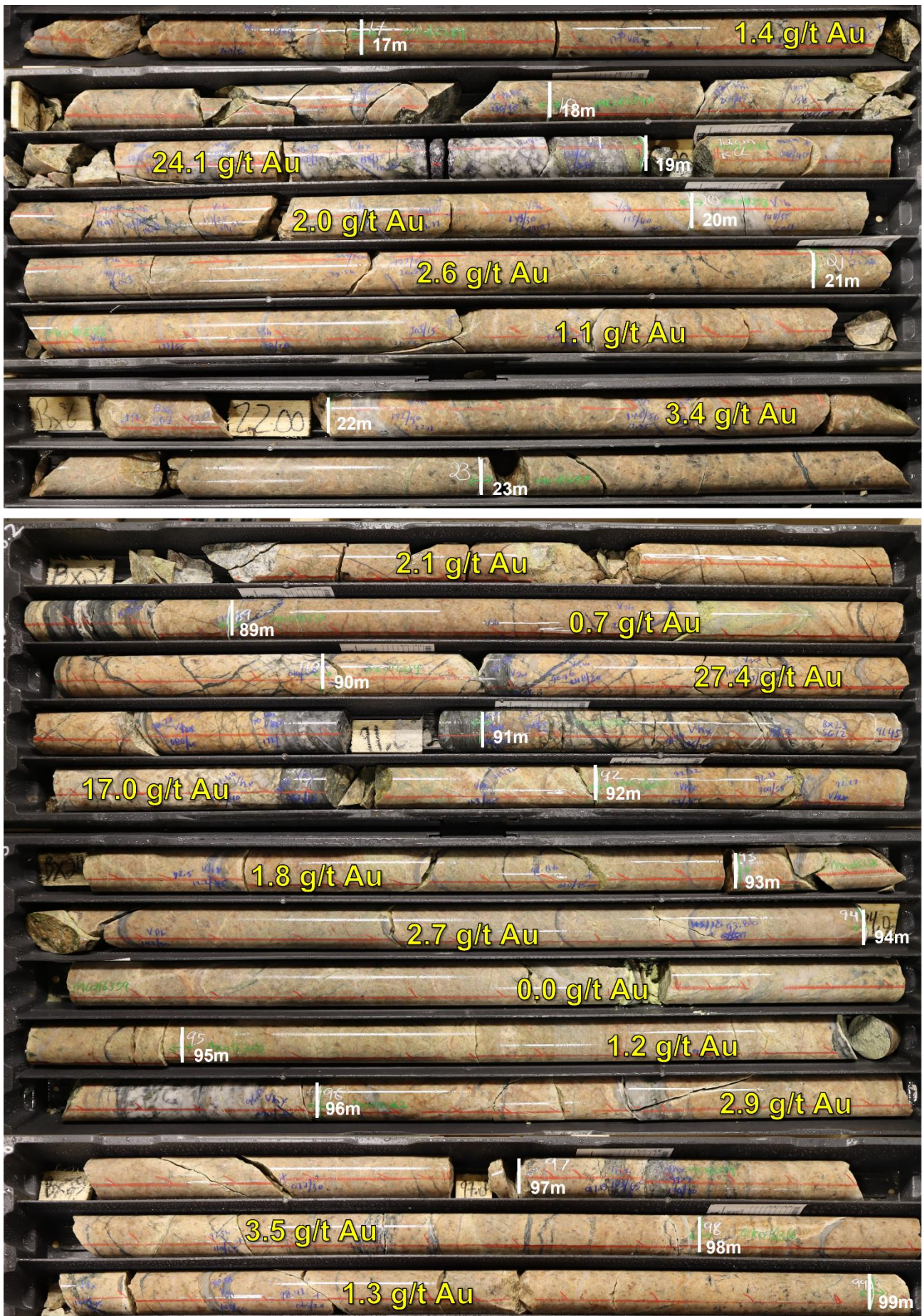
Figure 5: High grade gold association with increased density and width of sulphide-rich quartz stockwork and sheeted veins in CRD318
