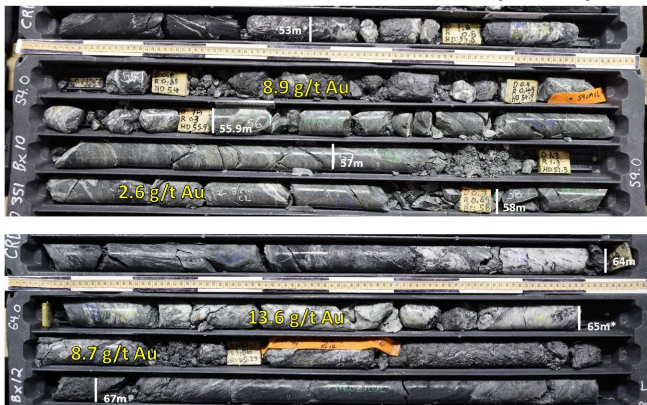
Figure 4: Detailed assays for CRD351 mineralised zone
