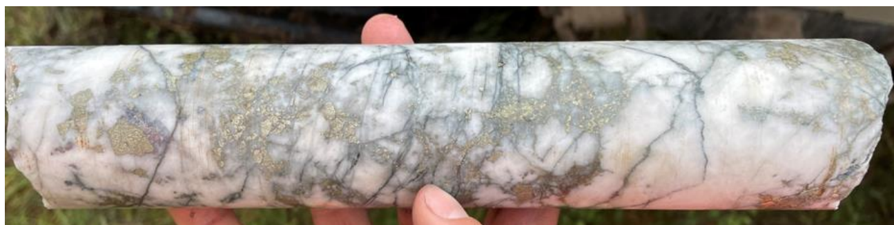
Figure 1: CRD212 - 1 metre @ 5 g/t Au in quartz-pyrite-galena veining (100-101 metres, within 22 metres @ 1.2 g/t Au from 91 metres)
