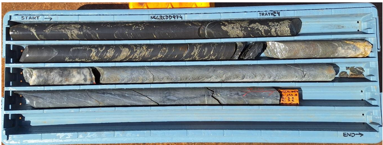
Tray 24 (249.91m – 253.11m) - Start shear zone, Raft of black shale, sheared and bleached mafic, quartz carbonate veins. Visible native gold in vein at 252m down hole. Veining and shearing continues.
