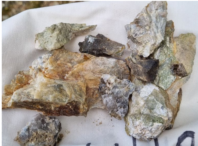
Figure 4: photograph of sample HLLH19 at Hälleberget that returned 0.13% Li 2 O with unknown lithium-bearing minerals
