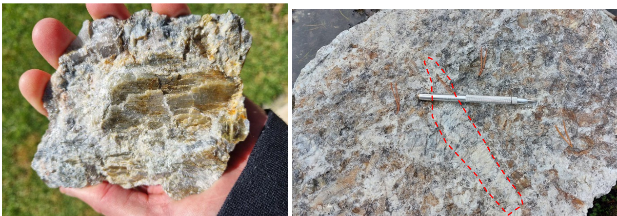
Figure 2: (left) Large 5cm by 3cm green spodumene crystals observed by Ragnar in boulders at the Orrvik prospect part of sample OVLH06 with assays of 1.2% Li 2 O. (right) outcrop rock sample observed by Ragnar showing 10cm long pale spodumene crystal (red outline) corresponds with sample OVLH14 and assays of 1.7% Li 2 O. See coordinates for all samples in Table 1.
