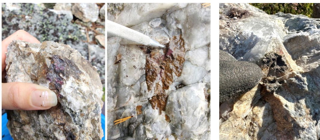
Figure 1: Dark to brownish triphylite-lithiophilite with purple heterosite-purpurite oxidation minerals at the Stenback spodumene prospect (left) compared to similar minerals at Dyngselet for sample BERG022 (centre) and Hälleberget for sample HALL038GS (right). See Table 1 for sample descriptions and locations.
