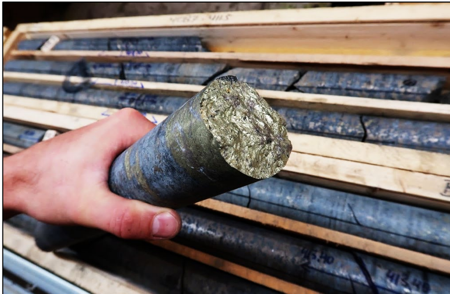
Figure 2: Chalcopyrite (Cu) rich vein at the top of the Lower Zone (409.4-409.6.m)
