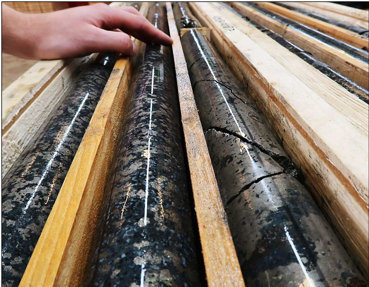
Figure 1: Close up of the pyrrhotite and pentlandite bearing Massive and Semi-massive (very coarse Interstitial) sulphides in the core of hole 22DDTS012 (405.8m-408.7m shown)
