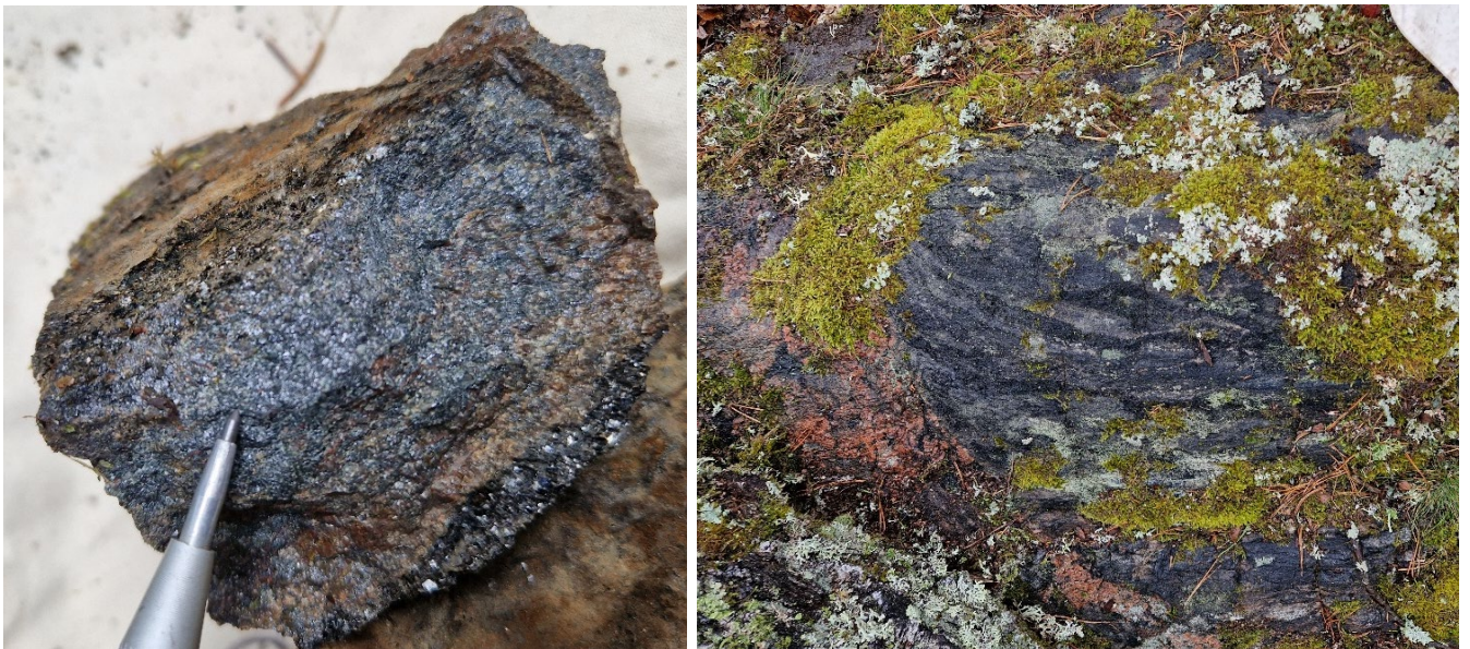
Figure 1: (Left) New discovery of biotite-magnetite-altered rock with 1.7% TREO (40% HREO) in B3739 at Melsjon; and (right) outcrop of biotite-magnetite-altered rock (black) with 4.1% TREO (40% HREO) in B3758 at Flaken.
