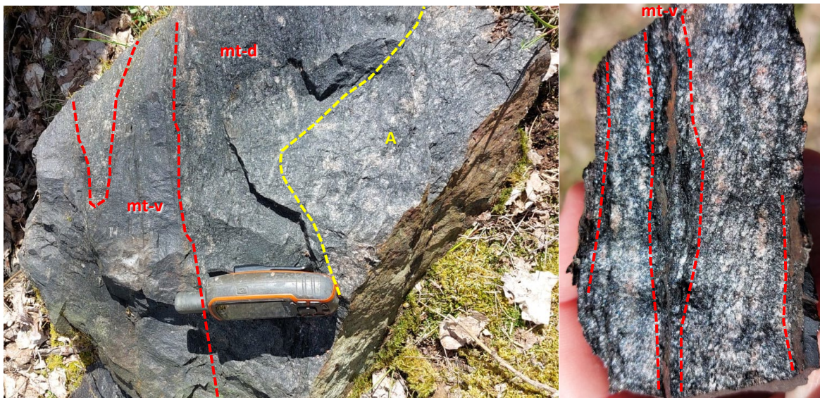
Figure 1A (left): Photograph of rock sample OLSGS003 with massive magnetite veins (mt-v) that returned 8,286 ppm TREO (86% HREE) as well as disseminated magnetite-altered (mt-d) augen gneiss (A). Figure 1B (right): Photograph of rock sample OLSGS001 of biotite-altered augen gneiss with magnetite (mt) veins that returned 9,012 ppm TREO
