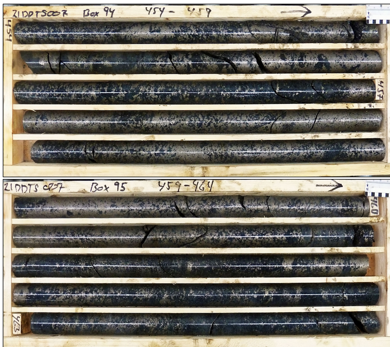
Figure 1: Magmatic Ni-Cu sulphides in 21DDTS007 displaying massive to semi-massive and matrix to coarse blebby sulphide mineralisation within the core of the host gabbroic intrusion (454m-464m shown)
