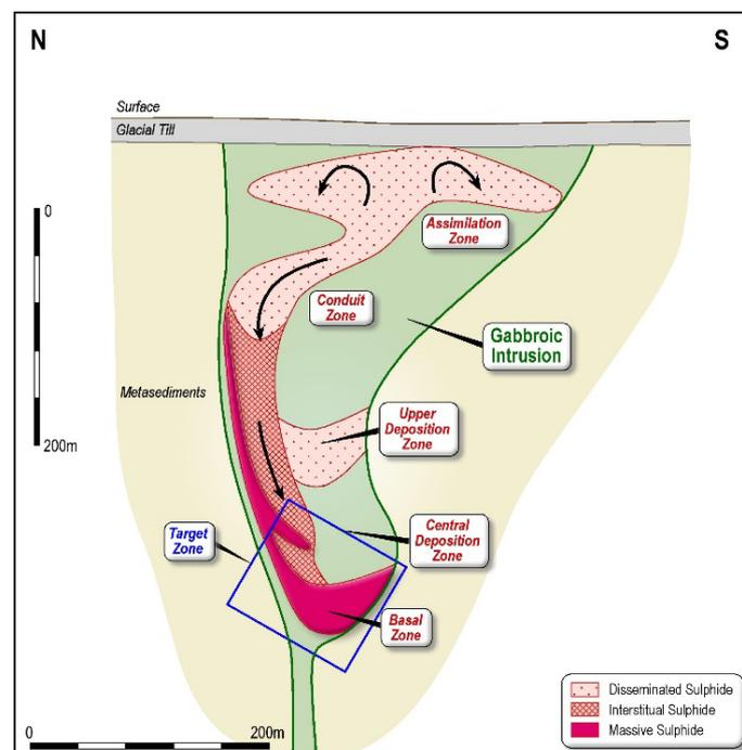
**Figure 3:** Schematic section showing the interpreted ore forming model within the Granmuren gabbro host intrusion. The Central and Basal zones are the most prospective for massive sulphide deposition and are the focus for future drill programs.
