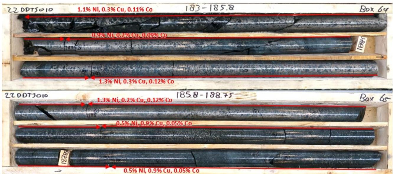
**Figure 1:** High tenor blebby, matrix and vein sulphide in the upper zone of hole 22DDTS010 showing assay results
