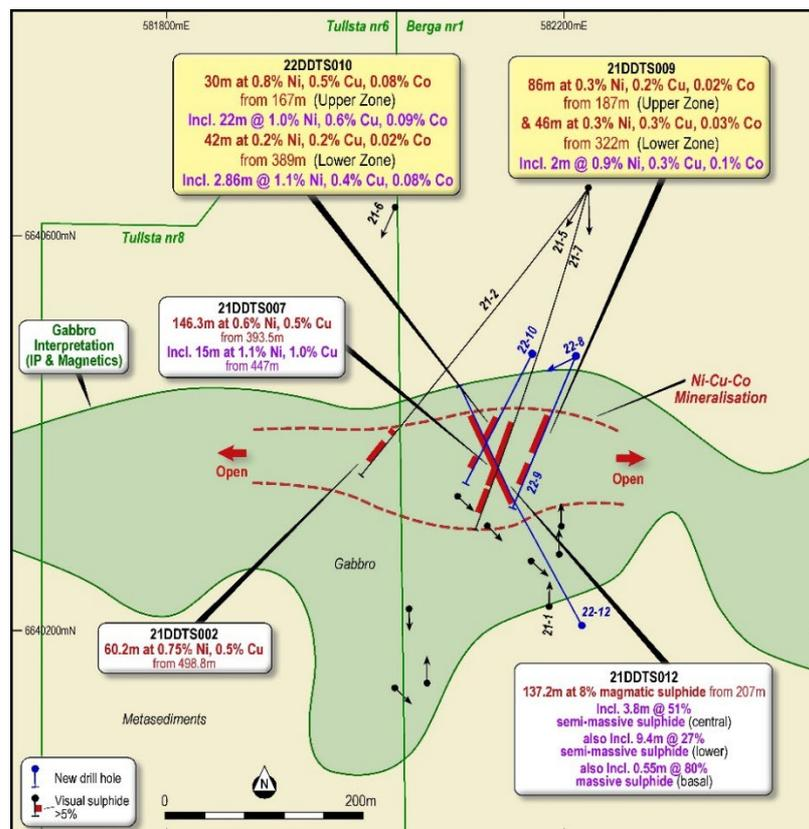
**Figure 2:** Simplified interpreted bedrock geology map of the host gabbro intrusion at Granmuren and highlighted drilling intersections.
