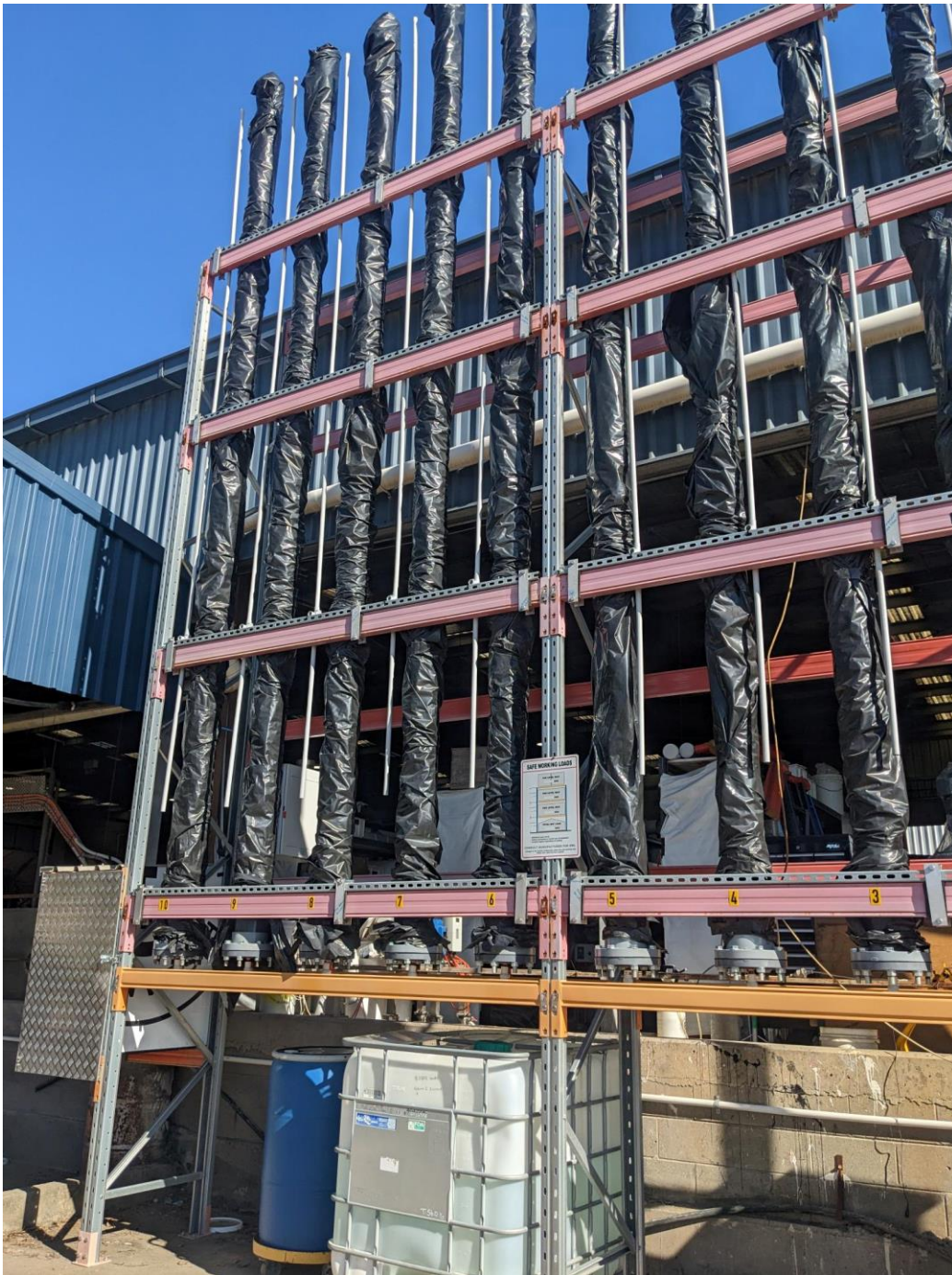
Figure 4: Column leach testwork on Dianne Copper Deposit material in progress
