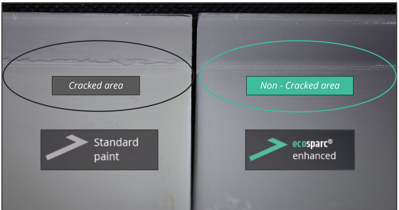
Figure 1: Significant improvement in crack resistance after 252 cycles of thermal testing
