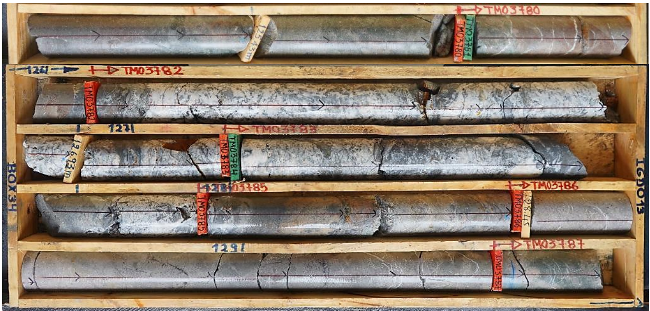
Figure 3: Mineralised intercept from drill hole IGD013, returning 2.69m @ 7.54g/t gold from 125.76m drill depth (image showing recovered core before sampling from 125.1m to ~130.6m depth).
