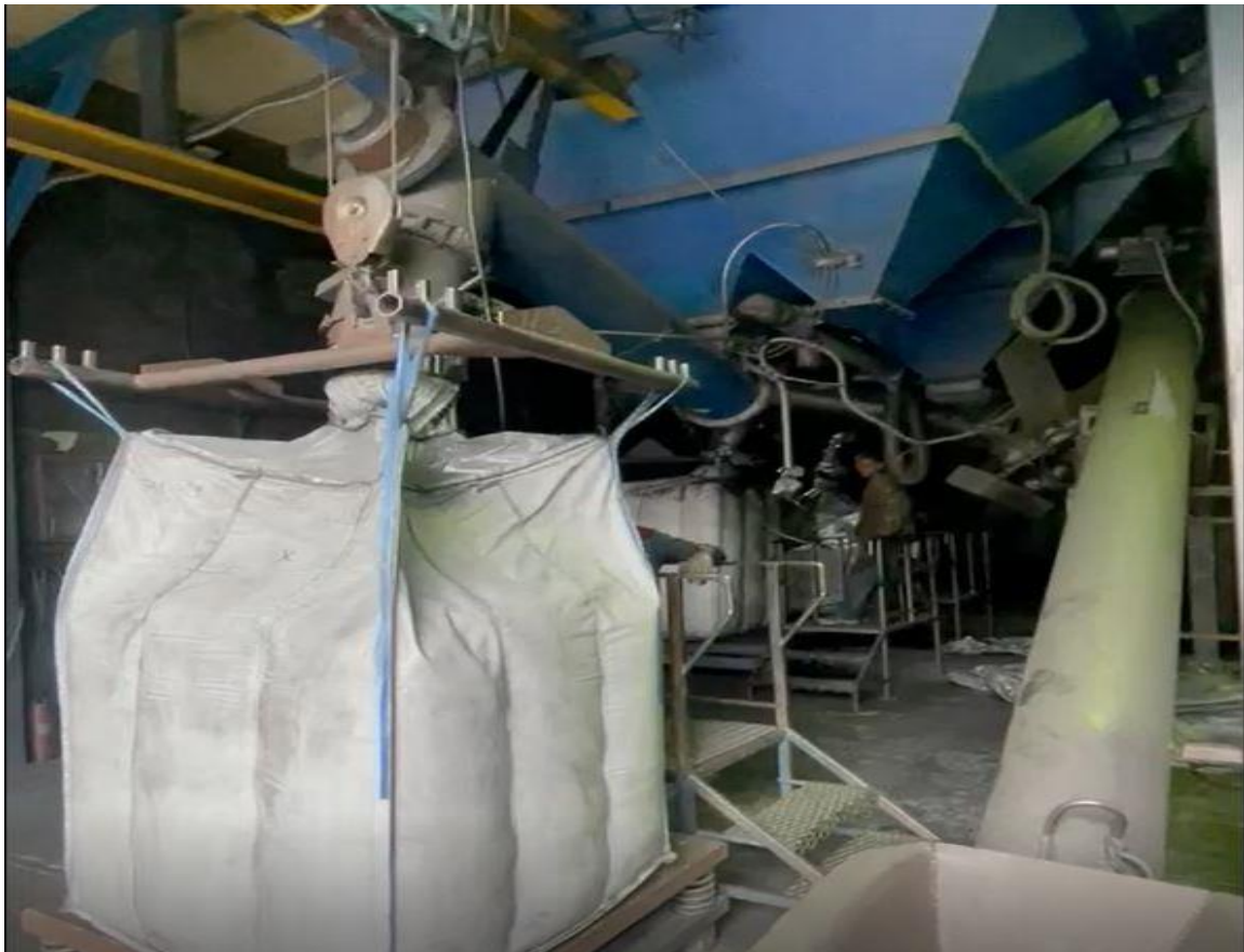
Filling bulk bag with graphite product
