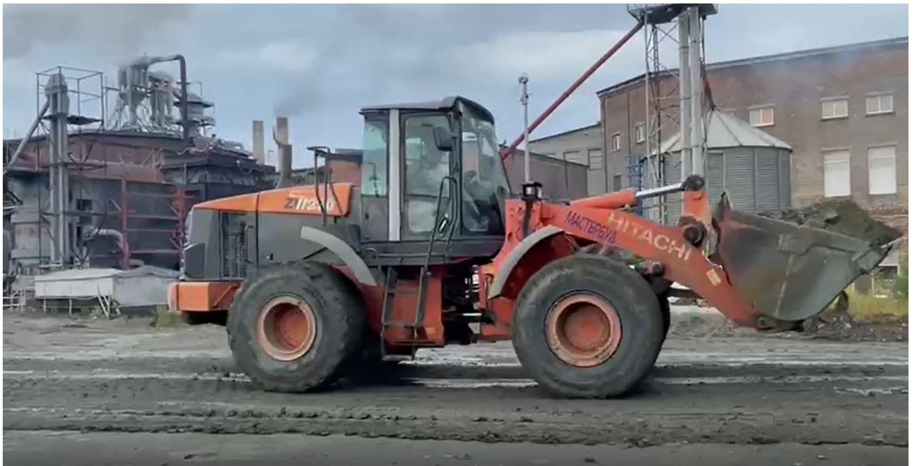
Tramming of plant ore feed from ROM stockpile to crushing circuit feed bin
