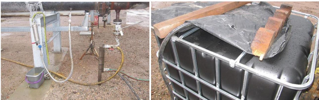
Figure 2: Photos of the geothermal well bulk brine sampling site and 1,000-litre bulk brine storage container.
